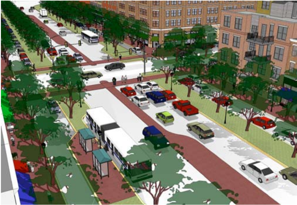
Left: New bus stops in the heart of the transformed Ethan Allen Gateway are visible in this view looking northbound on New Hampshire Avenue. Buses would travel in the through lanes and pull off at bus turnouts carved out of the side medians.
