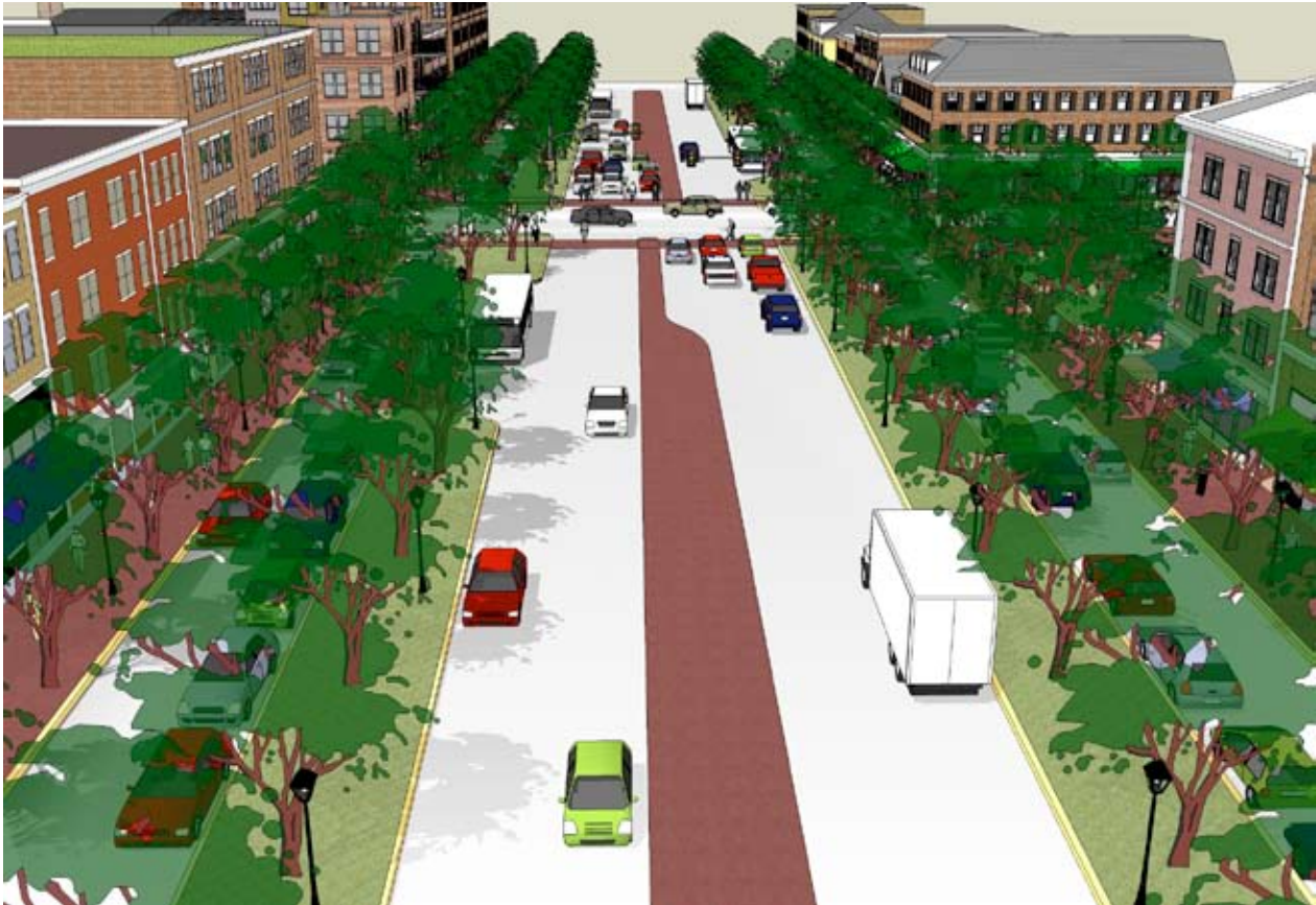
A computer-generated view looking southbound on a transformed New Hampshire Avenue. The changes balance access and transportation modes along the public right-of-way. The traditional user, the commuter vehicle , retains two through lanes with turning lanes at intersections. Buses have improved pedestrian access, ample bus stop facilities, priority light access and the option of upgrading the outer lane for bus use only as transit ridership builds. Bicycles will use the sheltered access lanes on the side - protected from fast moving traffic but with a clear shot across intersections, and the conversion to a wide shared-use trail along the wooded, non-commercial areas. Local vehicles are a secondary user in this access lane designed for slower cars, parked car access, and bicycles. Walkers gain access to half of the right-of-way: from bus shelters next to through-lanes across slow vehicle access lanes to businesses fronting on fifteen foot wide sidewalks.
